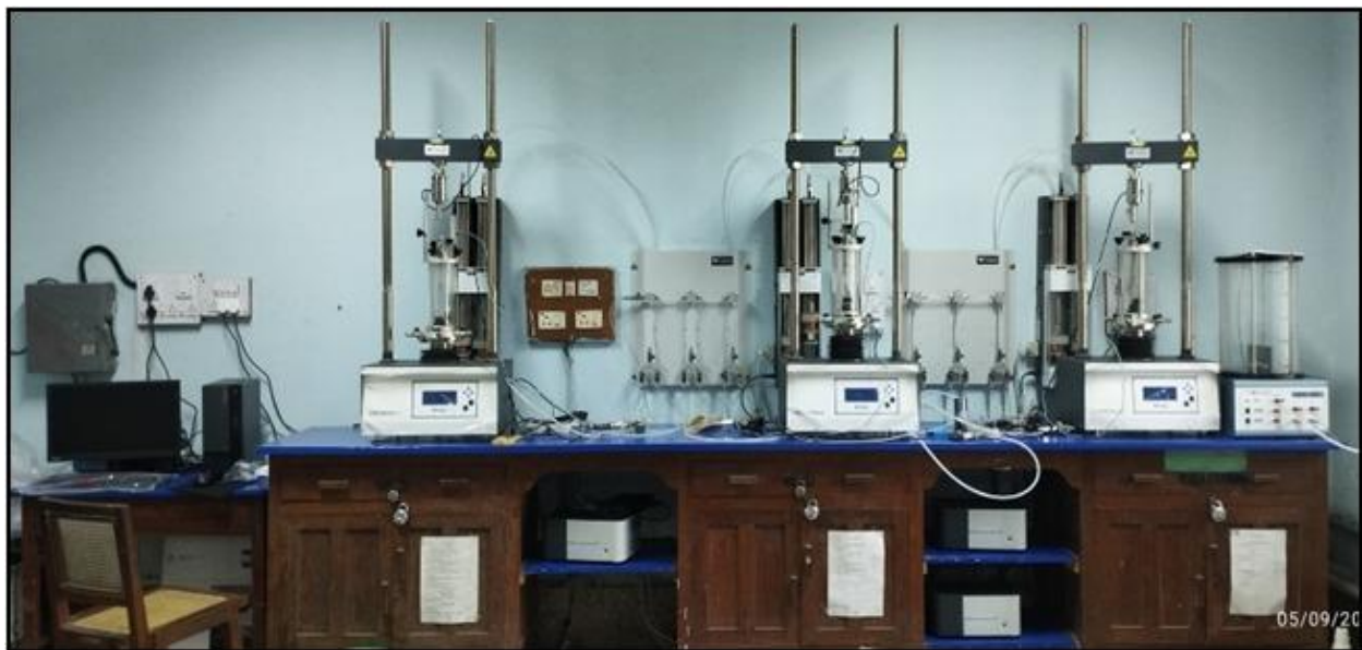
Figure 3.6 Triaxial shear test equipment
