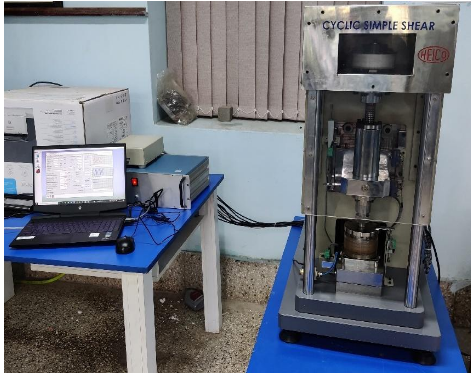
Figure 6.10 Laboratory cyclic shear test equipment
