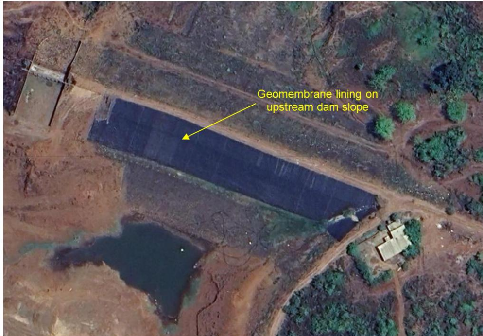
Figure 7.1 Upstream geomembrane lining
