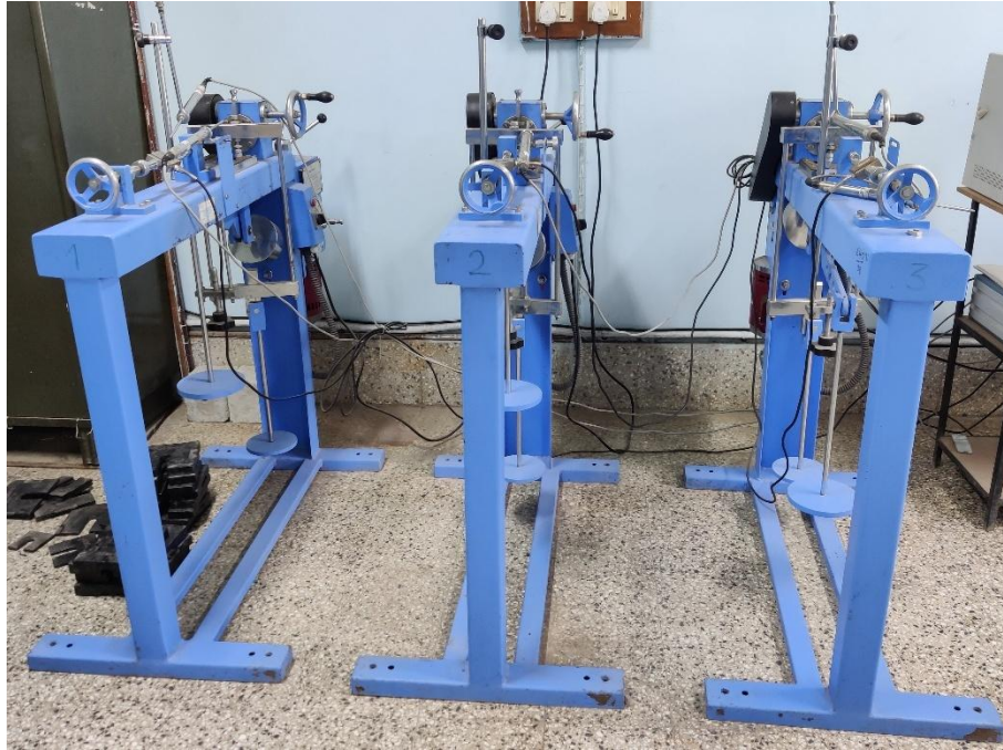
Figure 3.4 Direct shear test equipment
