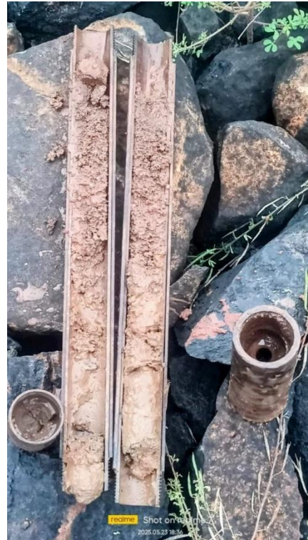
Figure 3.2 SPT test at dam site Figure 3.3 SPT split spoon sampler
