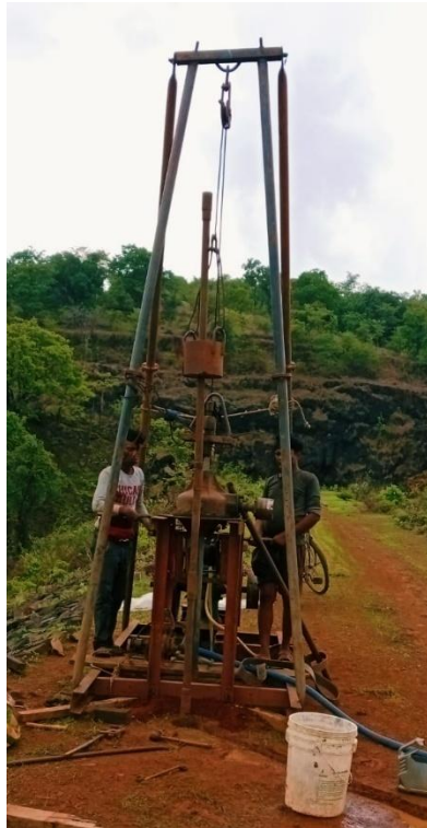
Figure 3.2 SPT test at dam site Figure 3.3 SPT split spoon sampler
